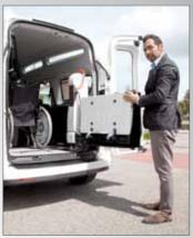
F-Twister® Allows rotating the Fiorella Lift by 90 degrees. This option makes loading of luggage and goods very easy, and it also represents a quick and efficient emergency exit. Not only! F-Twister also helps the caregiver to carry out wheelchair and occupant tie-down operation from a comfortable position, standing outside the vehicle.
