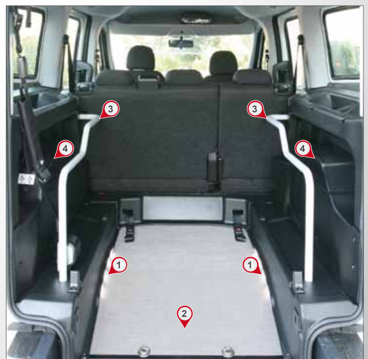
1 L.E.D. LIGHT KIT - 2 HIGH TECH FLOOR - 3 LEFT AND RIGHT SIDE HANDRAILS - 4 WHEEL ARCH COVERS
