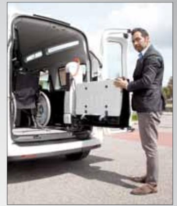
**F-Twister®** Allows rotating the Fiorella Lift by 90 degrees. This option makes loading of luggage and goods very easy, and it also represents a quick and efficient emergency exit. Not only! F-Twister also helps the caregiver to carry out wheelchair and occupant tie-down operation from a comfortable position, standing outside the vehicle.
